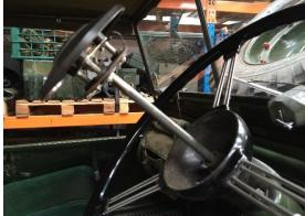
Undo and completely remove the steering wheel clamp holt
