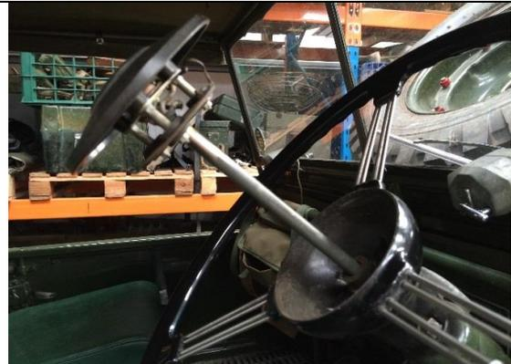
Undo and completely remove the steering wheel clamp bolt.
